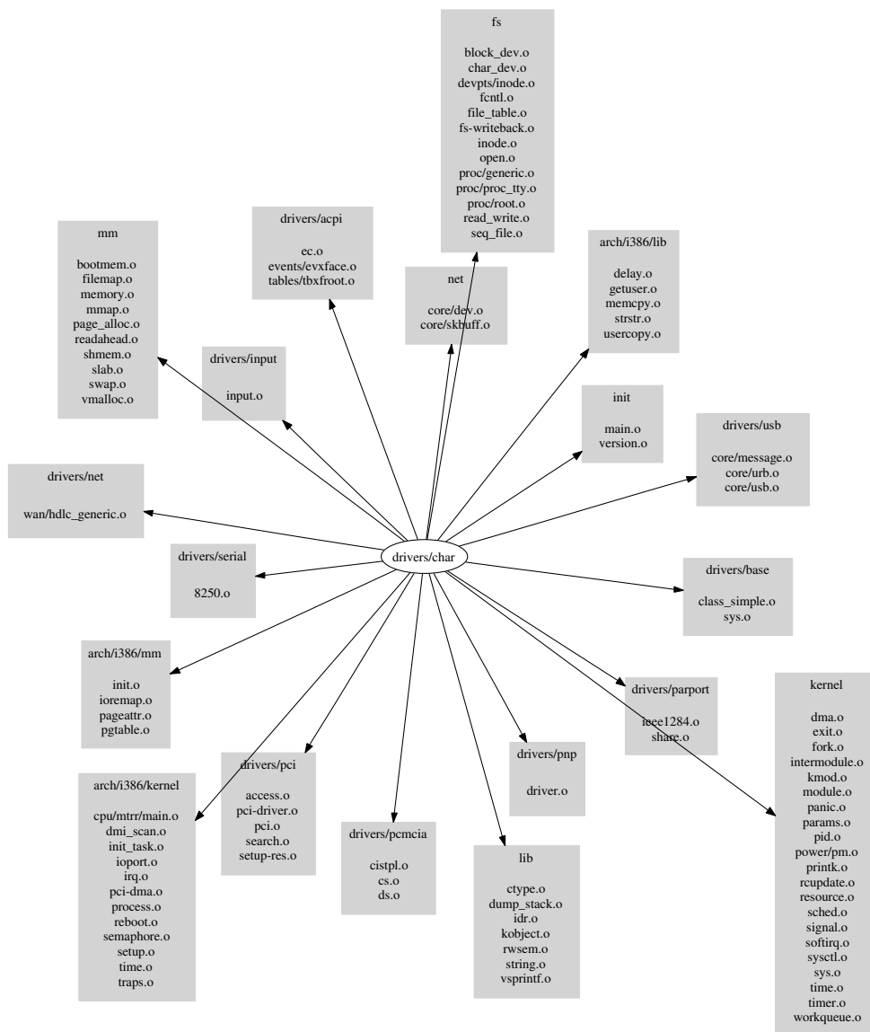
Figure 23: External dependencies of the drivers/char subsystem
